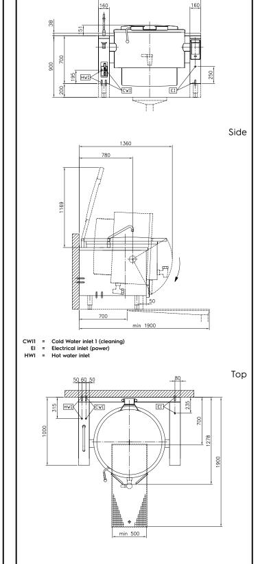
ProThermetic Sprint Electric Tilting Boiling Pan, 300lt Hygienic Profile, Freestanding
